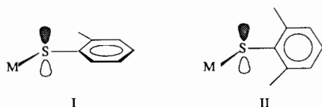
Fig. 3. Diagrams showing two conformations involving the orientation of aromatic ring with respect to the M-S-C plane.
